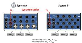
The combination of synchronisation and time stamp (TS) allows the clear allocation of signals that were captured by several systems.
