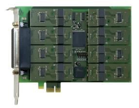
APCIe-7420 – 2-port serial interface RS232, RS422, RS485, 20 mA Current Loop
