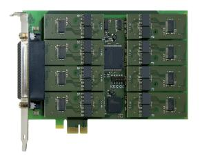
APCIe-7800 – 8-port serial interface RS232, RS422, RS485, 20 mA Current Loop
