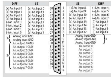
1: The analog inputs have a common ground line
