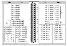
The analog inputs have a common ground line
